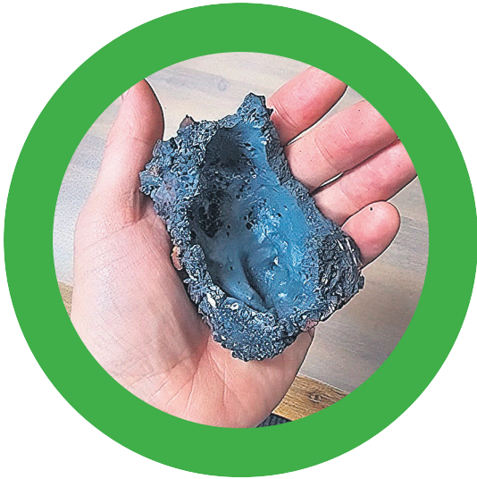
Metal Logic's first pig iron reduction test February 2023 (made from 55% Fe)
